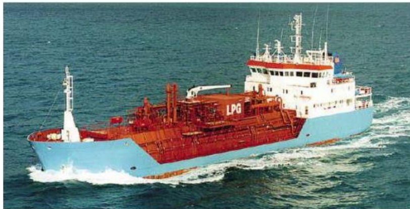
Figure 16. An example of a semi-pressurized LPG/NH 3 carrier.
