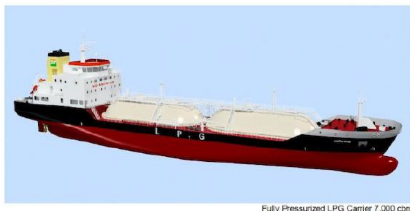
Figure 15. An example of a fully pressurized LPG carrier.
