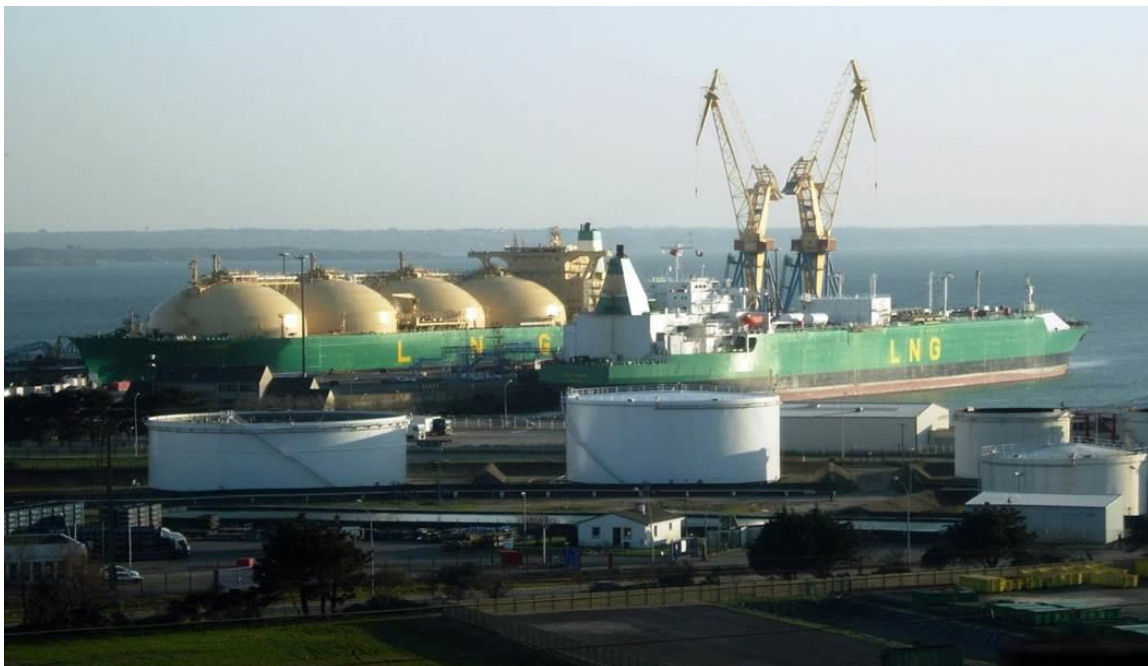
Figure 19 (Copyright Cedre). Overall view of a LNG carrier (Spherical type on the left, prismatic type on the right).
