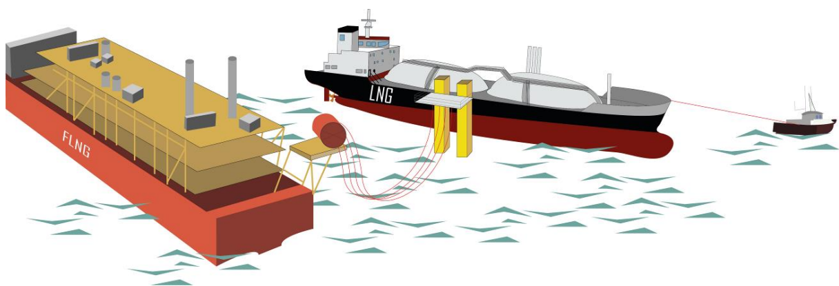
Figure 23 (Copyright Cedre). Tandem LNG offloading system. Reel (orange) holding flexible hoses for transfer operation).
