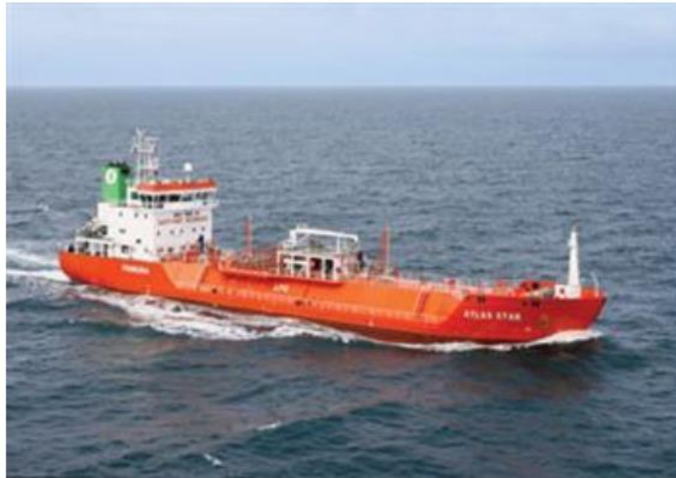
Figure 18. An example of a semi-pressurized/fully refrigerated ethylene/LPG carrier.
