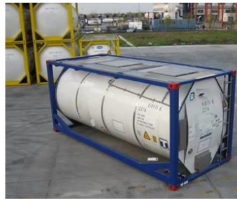
Figure 11. Intermodal tank containers: box type frame (left) and beam type frame (right).
